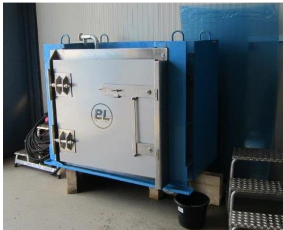
Test box after installation of the floodwater protection system in closed state
