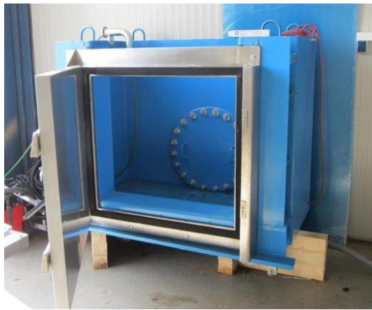
Test box after installation of the floodwater protection system in opened state
